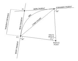
Chord - Any straight line connecting the tangents of a curve.
